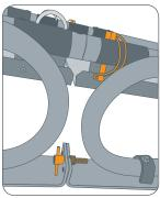
Tighten firmly the two knurled nuts on each toggle bolt.
